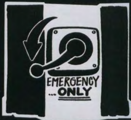
3rd Pull the emergency knob found near doors so that you can leave the doors open.
